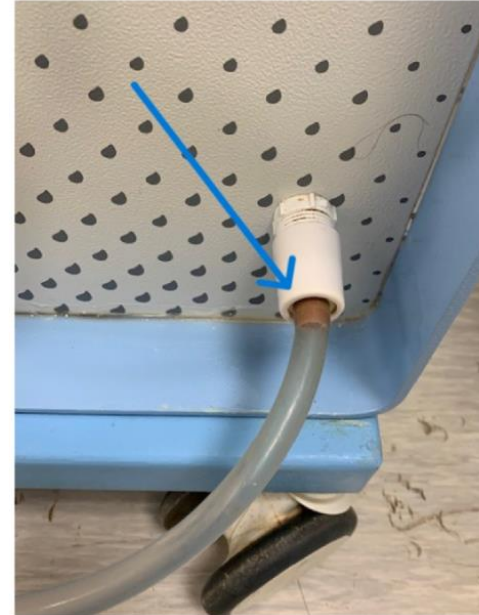
Fig. 1. Bath cart used to bed bath in intensive care unit patients with a specific reservoir to store and heat the no-rinse bathing solution, demonstrating visible dirt in the bath cart hose conduit and accumulation of dirt on bath cart connections.
